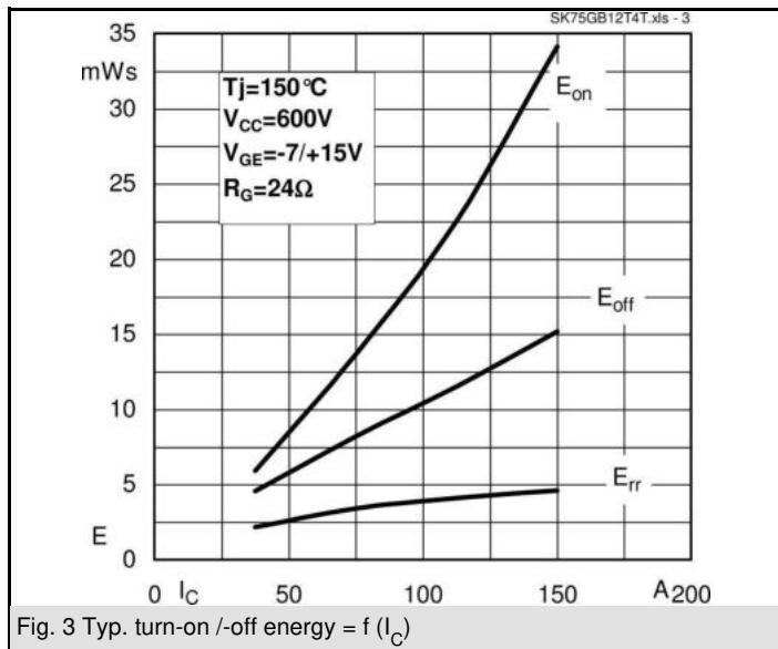
Fig. 3 Typ. turn-on /-off energy = f ( $I_C$ )
