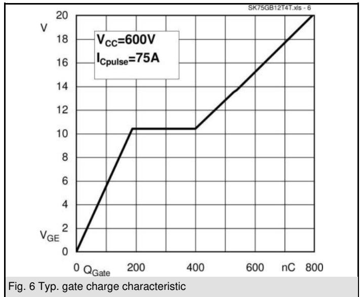
Fig. 6 Typ. gate charge characteristic
