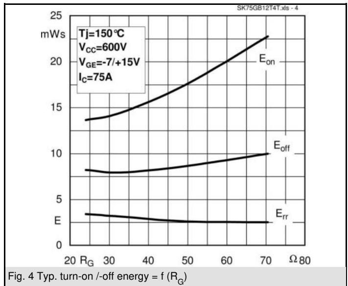
Fig. 4 Typ. turn-on /-off energy = f ( $R_G$ )
